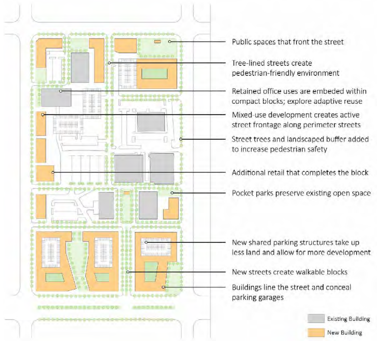
Figure 42: Potential Redevelopment of Typical Suburban Office Park
