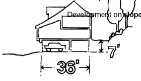
This home on a 15% uphill slope picks up grade by digging the garage into the hillside. Wide, shallow floor plans work better than deep plans on front-to-back slopes like this one.
