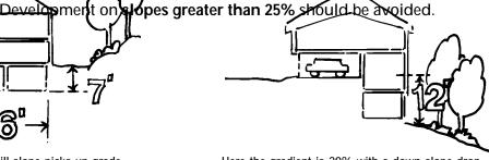
Here the gradient is 20% with a down-slope drop. A level, at-grade entry with volume built into the down-slope side of the house takes advantage of the grade change instead of fighting it.
