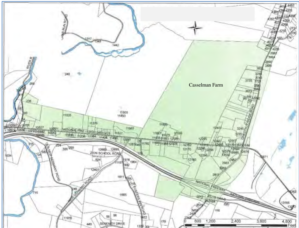
Figure 6.1: Expanded Water Service Area
