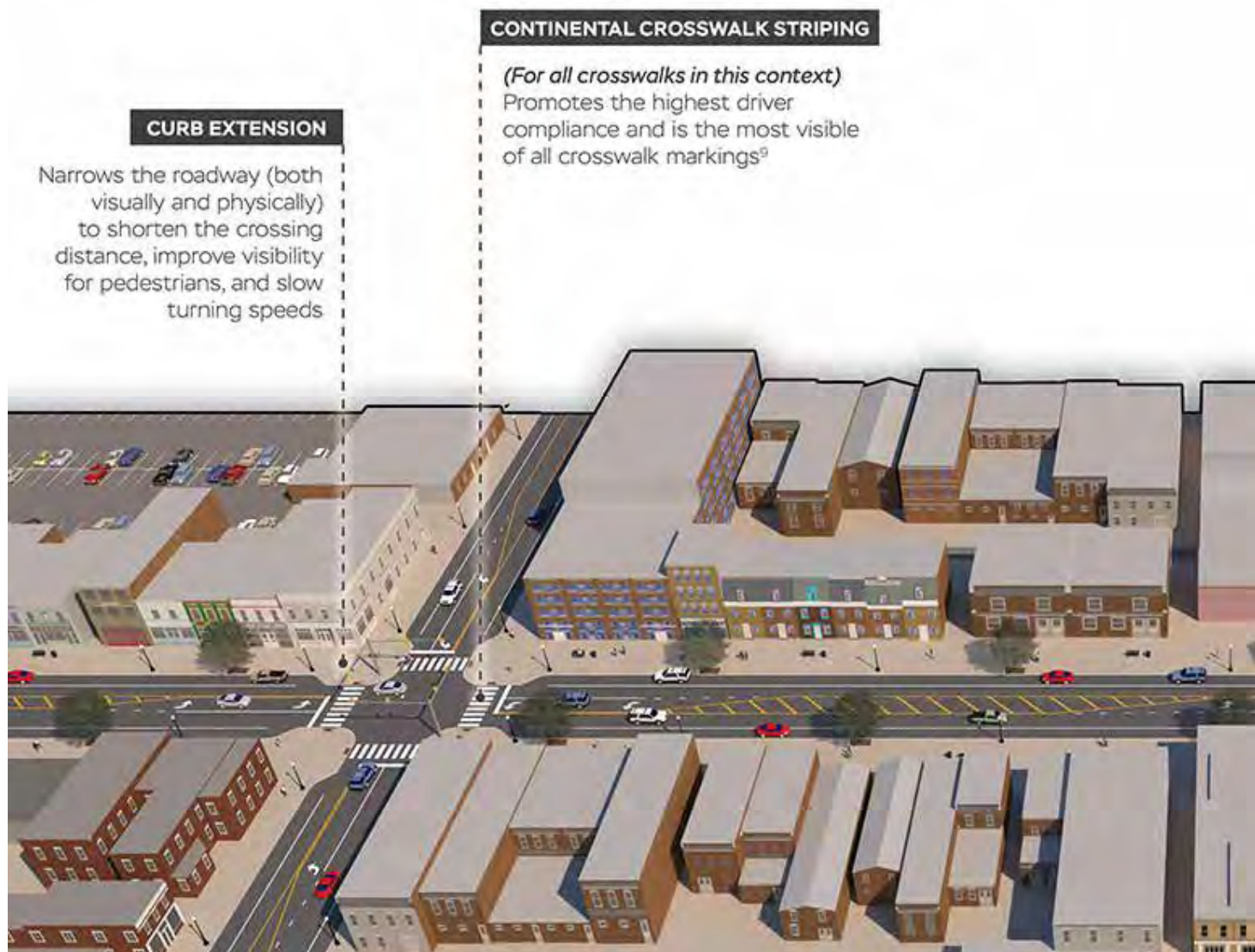
FIGURE 6-17: THROUGH A PLAN CALLED 'CONTEXT DRIVEN: ACCESS AND MOBILITY FOR ALL USERS', MDOT/SHA HAS CREATED A SET OF PROTOTYPICAL MARYLAND ROADWAY CONTEXTS WITH TAILORED RECOMMENDATIONS TO IMPROVE SAFETY. THE EXAMPLE ABOVE SHOWS THE 'TRADITIONAL TOWN CENTER' CONTEXT WHICH IS BROADLY APPLICABLE TO MOST OF ANNAPOLIS' MOST DANGEROUS ROADWAYS
