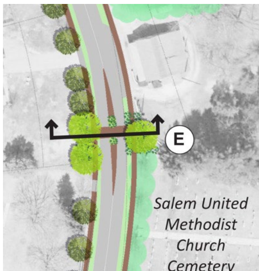
Figure 27 - High Street Transition illustrating the use of a splitter island as a traffic calming measure as well as a refuge island to protect pedestrians in the proposed crosswalk
