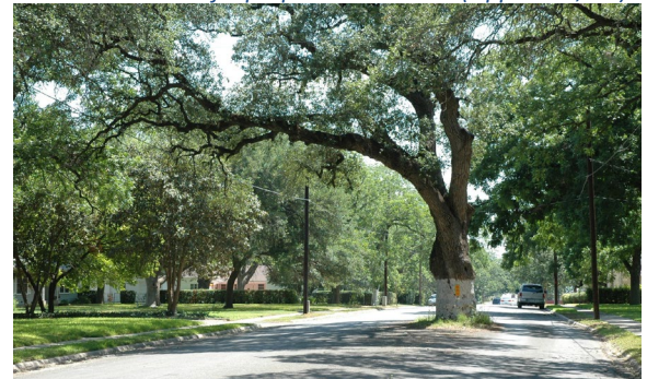
Figure 16 - Use street trees in both gateway and transition areas to enclose driver views and increase "visual friction" (Source: https://howwedrive.com/2008/08/17/natural-traffic-calming/ )
