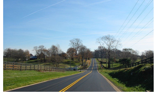
Figure 14 - Flush curbs in gateway areas clue drivers that they are entering a settled place (Upperville, VA)
