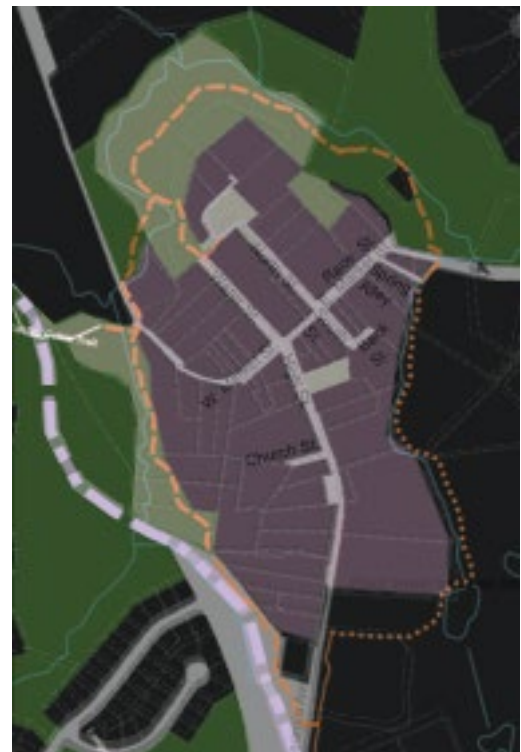
Figure 23 Conceptual diagram of natural surface trail utilizing existing parkland and public right-of-way (long dashed line). Trail easements would be required along the stream valley from Manor at Silo Falls to Brighton Dam Road (short, dashed line)
