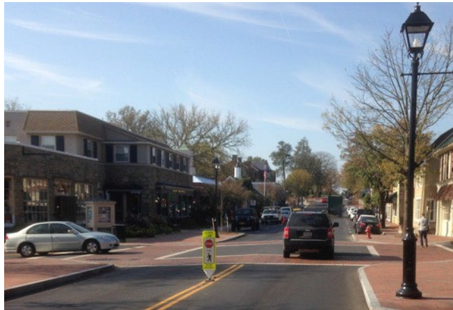
Figure 34 - Use of vehicular clay pavers (crosswalks), granite curbs, traditional brick pavers (sidewalk) and historically appropriate light fixtures (Middleburg, VA)
