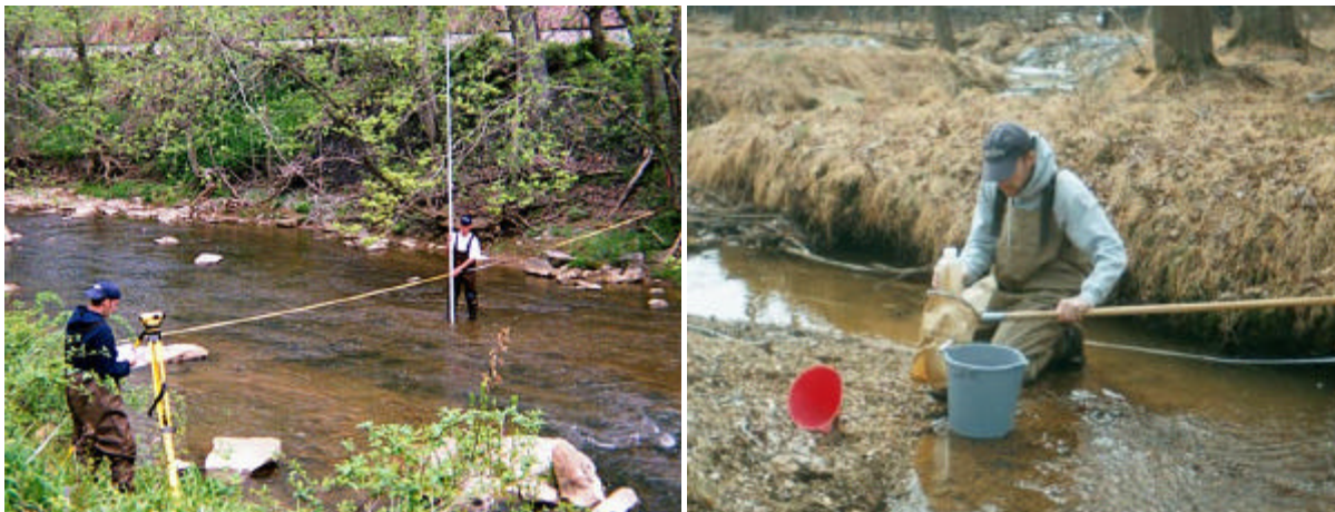
Figure 3 Important components of stream monitoring, habitat assessment (on left) and benthic macroinvertebrate sampling (on right), help to determine the physiological and biological health of a stream. These characterize stream health and water quality under present conditions and establish a baseline for evaluating future conditions as new developments are built.
