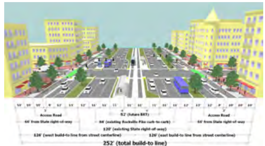
2016 Rockville Pike Neighborhood Plan Multi-Way Boulevard Typical Street Section. This street section is not expected to be fully realized along Rockville Pike due to space constraints and design exceptions.
