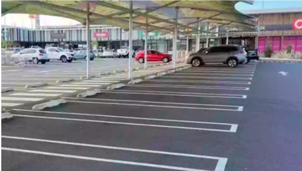
Parking spaces with double-lined markings.
