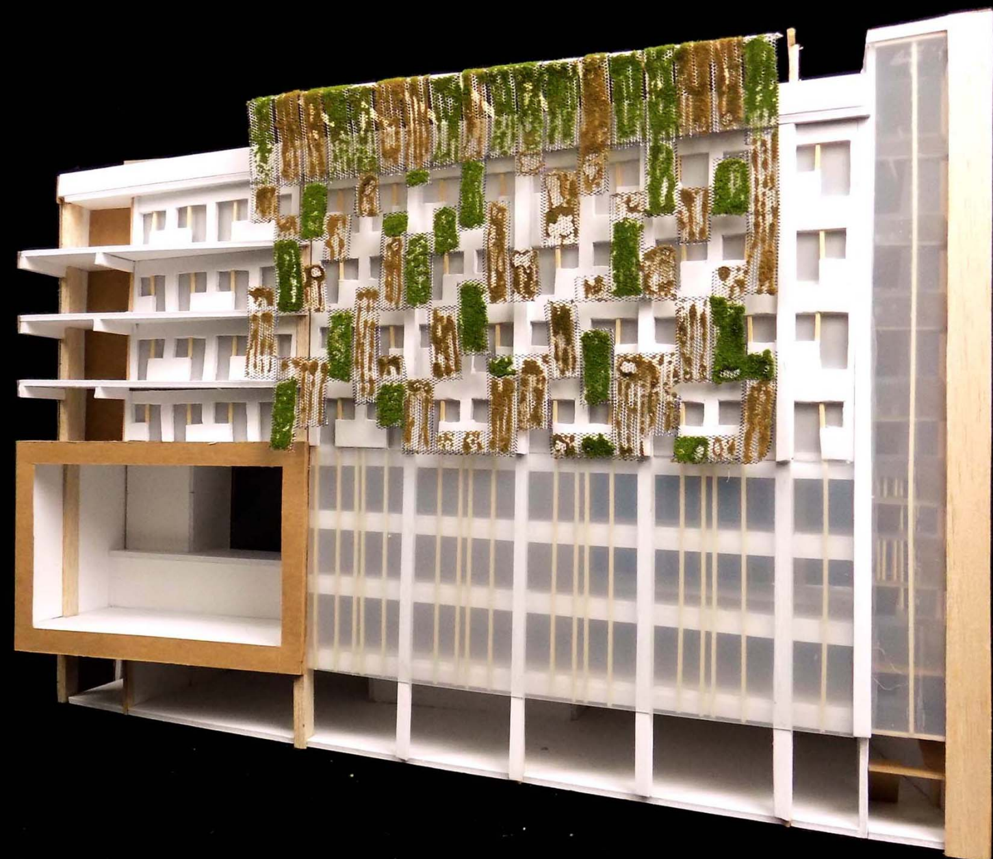
View of 1/8” Scale Model South-facing Facade, including “Green Skin,” Curtain Wall, and Public Performance Area
